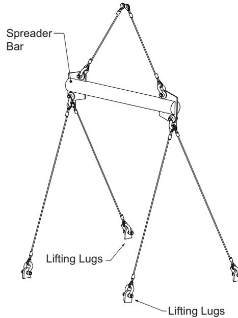
PCUs ordered with or without a KB fan all come with quantity four [4] lifting lugs factory installed on the four [4] corners of the unit. **Figure 2** illustrates a PCU with a KB fan attached.
