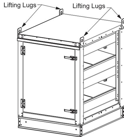
PCUs ordered with a USBI or SIF fan still include quantity four [4] lifting lugs factory installed on the four [4] corners of the PCU filter module assembly which must be used as the primary method of lifting the unit (**Figure 4**). Additional lifting points should be used in the below priority:
