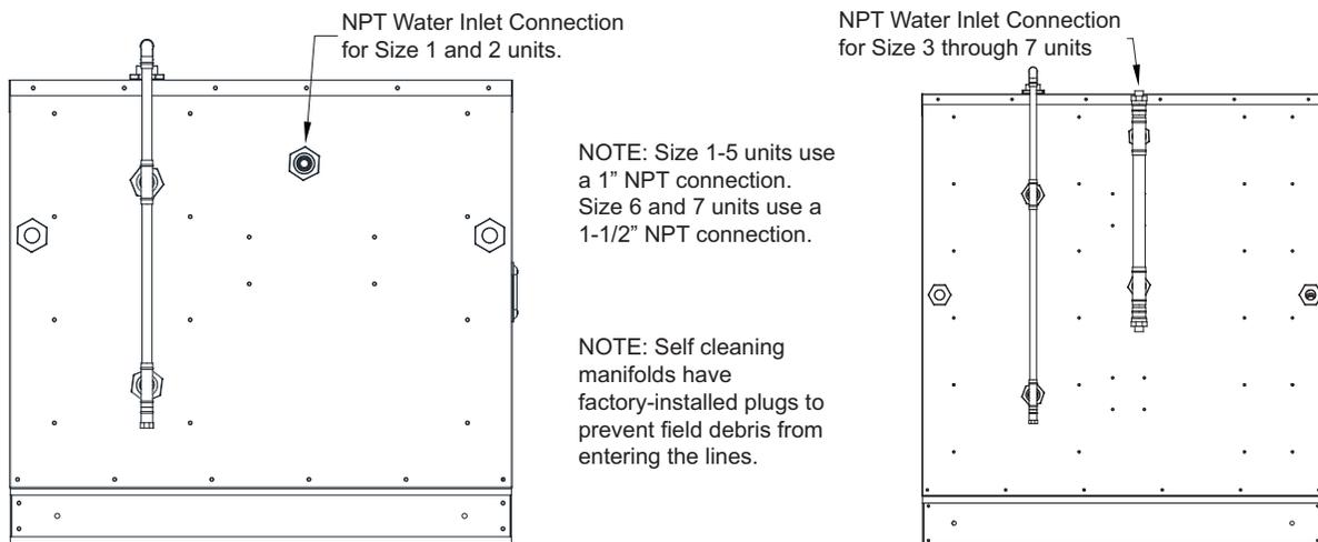
**If the PCU is mounted outdoors, heat tape must be applied to all external piping for the ESP Self-Cleaning System (SCS). If a self-draining SCS package is used, heat tape is not necessary.**
