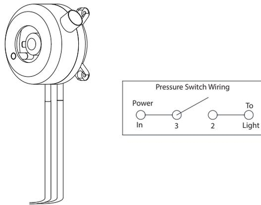
**Figure 11 - Airflow Switch Installation**
