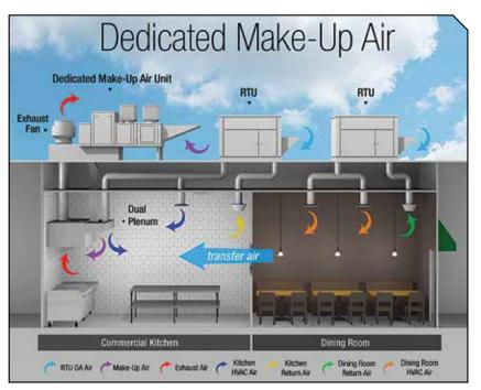
FIGURE 1. Ventilation system schematic with dedicated makeup added.
