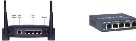
Figure 6 - Wireless Router/Ethernet Switch
