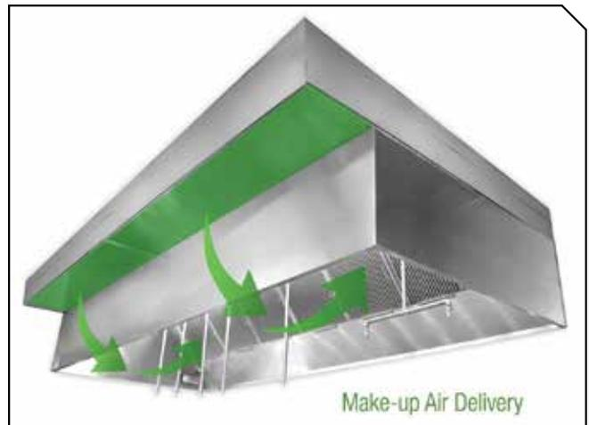
**FIGURE 2.** Wall canopy hood with single plenum perimeter makeup air distribution device.
