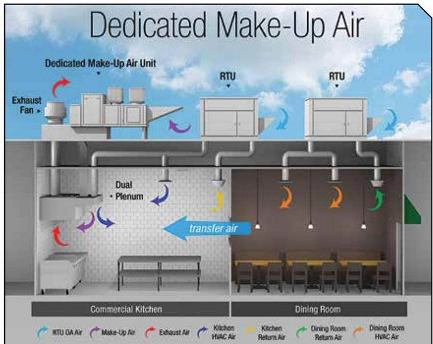
**FIGURE 1.** Ventilation system schematic with dedicated makeup added.
