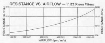
Average arrestance is 54% at 350 fpm when tested per ASHRAE 52-76 testing procedure.
