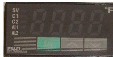
There are two factory set ranges of temperature controls. The low temp range is factory programmed for 400-450°F rated hoods. It is pre-programmed to turn the fans on automatically at 85°F and to send the fans to high speed at a 90°F duct temperature. The high temp range is factory programmed for 600-700°F rated hoods. It is pre-programmed to turn the fans on automatically at 85°F and to send the fans to high speed at a 130°F duct temperature.
