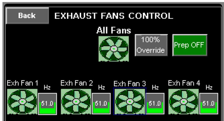
The fans take a few seconds to come up to speed. The VFDs should all indicate **48Hz** and the **All Fans** indicator light should be green and "turning". This indicates that the fans are operating on low speed. If the supply fan drive does not ramp up, verify that there isn't a fire Condition Alarm on the Touch Screen. If that's the case, the fire system might be tripped or not properly wired.
