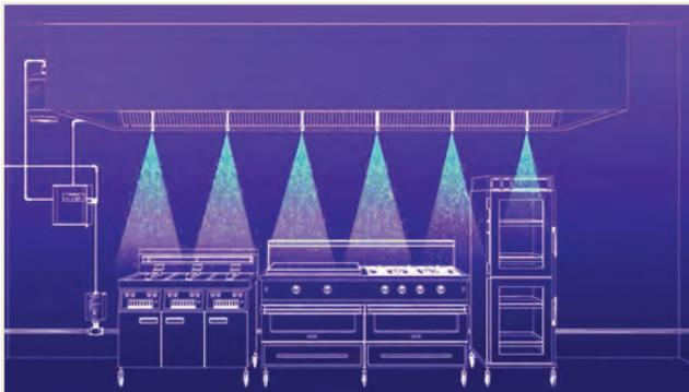
FIGURE 4: Overlapping pipe and nozzle design.
