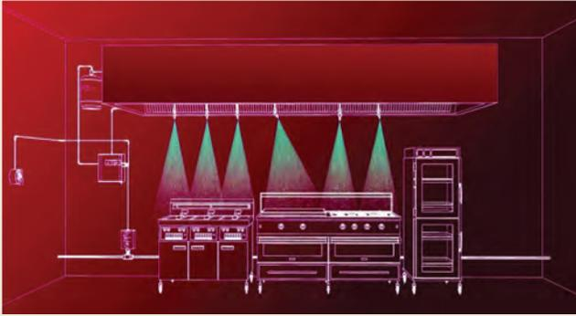
FIGURE 3: Appliance-specific pipe and nozzle design.
